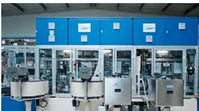
Assembly system for the joining elements for exhaust pipes in Gerbershausen
