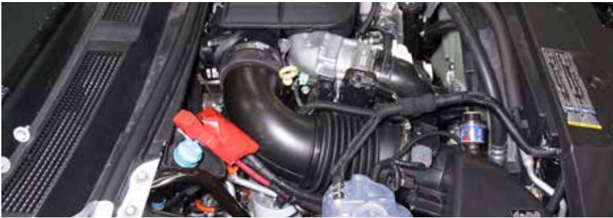
TWIST III VO SP , welded on a blow molded pipe
